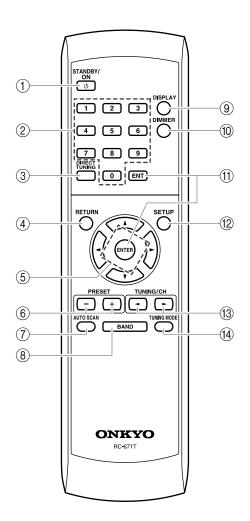
1 STANDBY/ON button (15) Sets the T-4555 to On or Standby.
